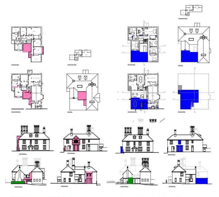
Existing floor plans and elevations showing demolitions
